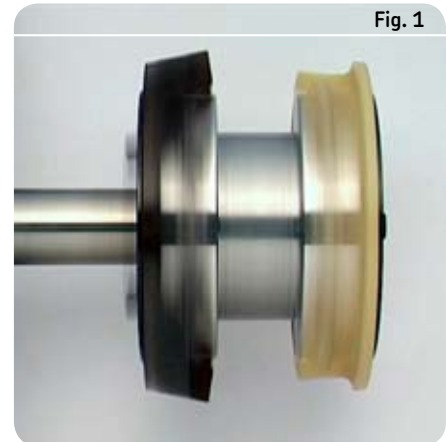
Fig. 1 A polyamide cage from a standard SKF bearing and an E2 bearing are running at 8 000 r/min. The E2 cage on the right shows significantly less deformation.
