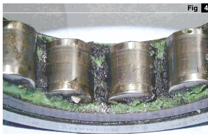
Black discoloured grease affected by current discharges
