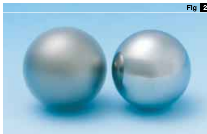
The dull surface of the ball is a sign of micro-cratering
