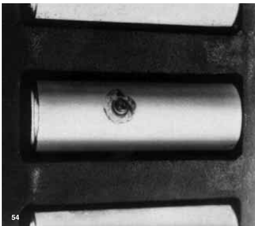
Fig 54 Roller of a railway axlebox bearing damaged by electric current (same bearing as in fig 53)
