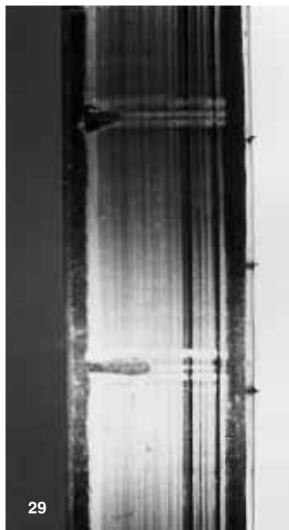
Figs 28–30 An example of the results of improper handling. A roller in a double row cylindrical roller bearing has suffered impact (fig 28). A periphery camera view of the roller shows two diametrically opposed indentations (fig 29). The roller has, in turn, dented the inner ring raceway (fig 30)
