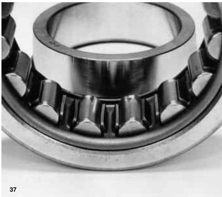
Fig 37 A cylindrical roller bearing with smear streaks in the inner ring raceway and on the rollers. The smearing has been caused by the roller assembly being entered askew without being rotated
