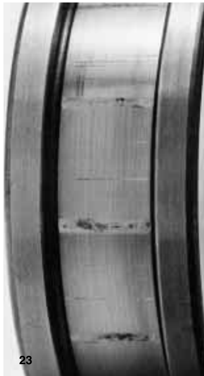
Fig 22 Outer ring of taper roller bearing damaged by vibration during operation
