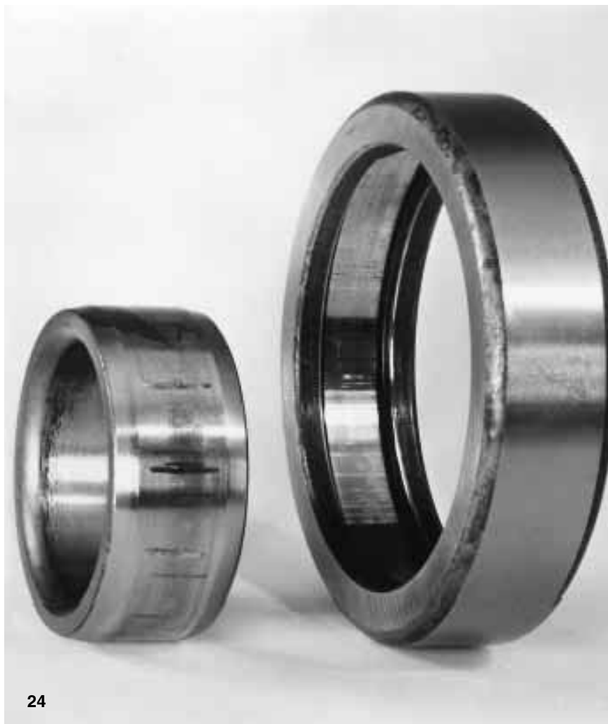
Fig 26 Outer ring of a self-aligning ball bearing damaged by vibration. The bearing has not rotated at all
