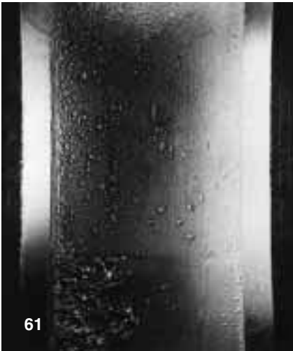
Fig 61 Cylindrical roller bearing inner ring with flaking at one side of the raceway, as a result of overloading due to misalignment
