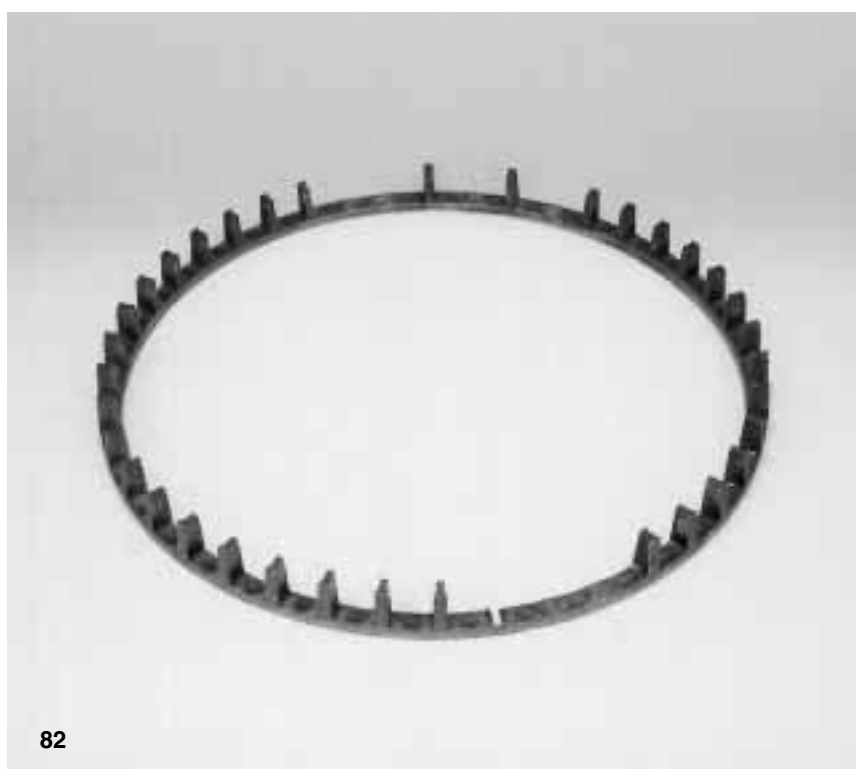
Fig 82 Cage of a spherical roller bearing. Fatigue cracks have formed in the fillets
