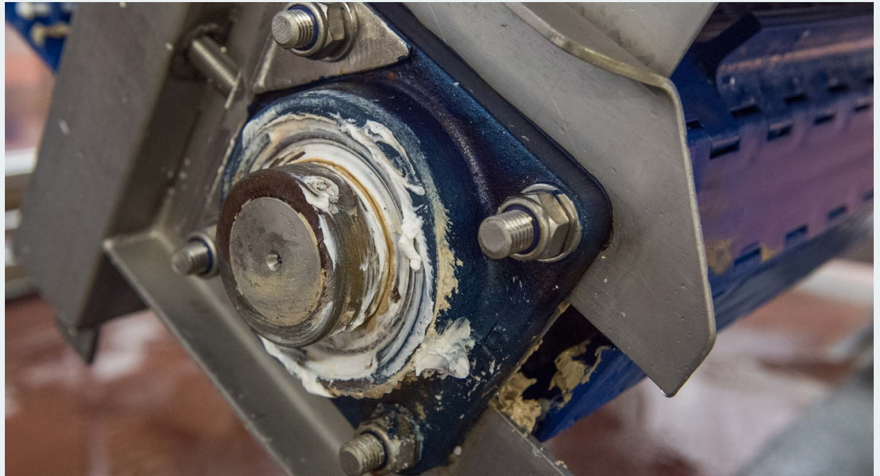
Excess grease from the bearing has collected on the hygienic conveyor belt, increasing the potential for bacteria or allergens to enter the food zone and compromise food safety.
