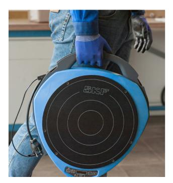
Utilizing electrical power, the TWIM 15 features glass-fiber, high-temperature-resistant plastic construction that allows a low temperature difference between the inner and outer rings of the bearing. This helps to reduce internal tensions that are generated due to excessive thermal expansion of the inner ring compared to the outer ring.
