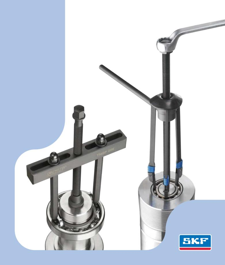
The SKF Deep Groove Ball Bearing Puller Kit TMMD 100 allows quick and easy dismounting of SKF Deep Groove Ball Bearings with an interference fit on both rings.
