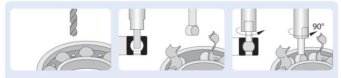
Remove seal and open selected section of ball cage. Clean the swarf out.
