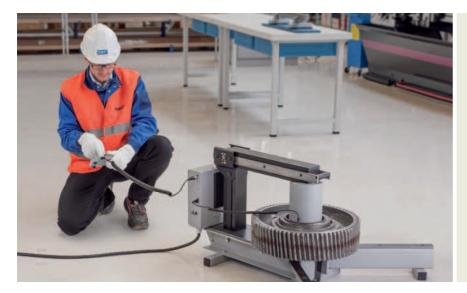
The TIH L MB induction heater is equipped with a remote control panel for operator safety.
